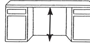
1. Measure height of cabinet opening from underside of countertop to floor.
