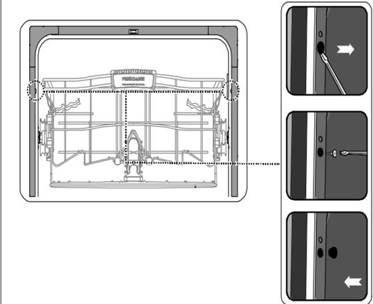
14. Open and close dishwasher door slowly. Ensure that there is clearance to the console. Adjust accordingly until door opens and closes freely.
